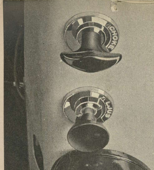
Parking lights (Lighting switch pulled out one notch)
